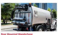
**Rear Mounted Wanderhose** for catch basin suction and drain clearance with pendant control to aid the operator.
