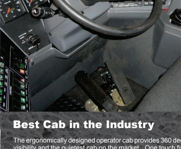
The ergonomically designed operator cab provides 360 degree visibility and the guietest cab on the market. One touch finger controls minimize operator fatigue during a snow event. Dual thermal pane glass with electrically heated windows ensure the operator has the best visibility in all conditions
