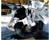
The new broom design revolutionizes the application of brooms for airport use. The wafer broom exceeds all performance criteria during a snow event. The 22ft, 35 degree angle, 46 inch diameter broom, with wafer bristles, puts the power to the surface with increased broom rotation speeds. Only two castor wheels are necessary each 31 inch in diameter, with mechanical turning adjustments, supporting higher operating speeds, with no castor wobble.
