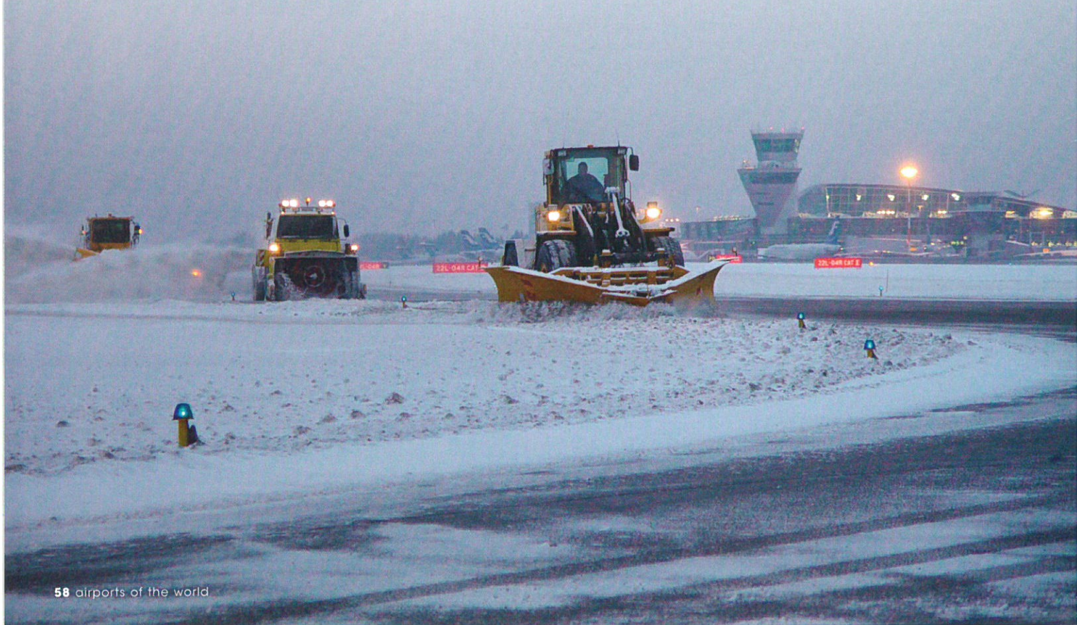
▼Tractor units with ploughs clear runway and taxiway edges where lights stand proud of the surface. (Finavia)
