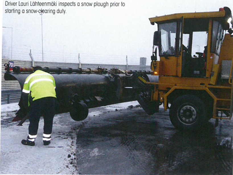
Ploughs are fitted with independent spring-loaded cutting segments to clear uneven surfaces
