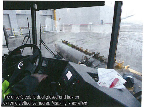
Each Vammass PSB 5500 has a plough, brush and snow blower. (Finavia)
